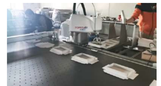
纸盒包装: 31pcs/min 精度正负0.3mm Carton packaging: 31pcs/min, accuracy plus or minus 0.3mm
