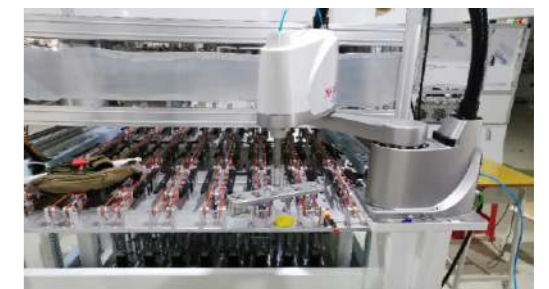
下料机: 传感器 (4条传送带, 8s) Unloader: Sensor (4 conveyor belts, 8s)
